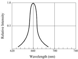
Fig.1 RELATIVE INTENSITY VS. WAVELENGTH
