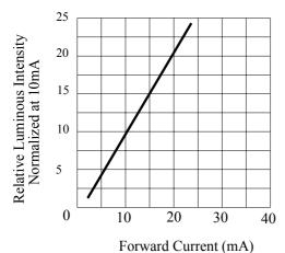
Fig.5 RELATIVE LUMINOUS INTENSITY VS. FORWARD CURRENT
