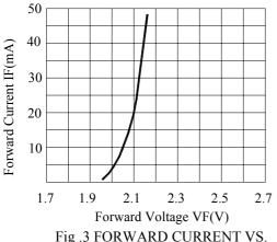
Fig .3 FORWARD CURRENT VS. FORWARD VOLTAGE PER CHIP
