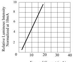
Forward Current (mA) Fig. 5 RELATIVE LUMINOUS INTENSITY VS. FORWARD CURRENT
