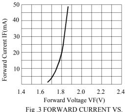
Fig .3 FORWARD CURRENT VS. FORWARD VOLTAGE PER CHIP
