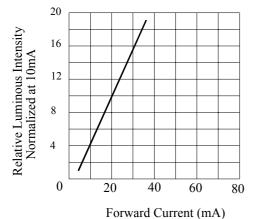
Fig.5 RELATIVE LUMINOUS INTENSITY VS. FORWARD CURRENT
