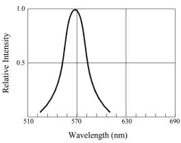
Fig.1 RELATIVE INTENSITY VS. WAVELENGTH
