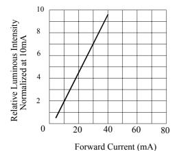
Fig. 5 RELATIVE LUMINOUS INTENSITY VS. FORWARD CURRENT
